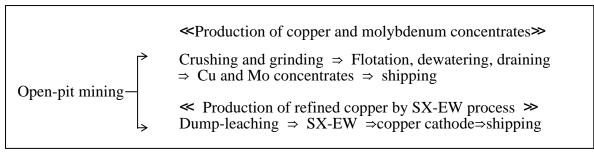
Notes 1: (1)Dump-leaching means a process to extract (leach) copper by sprinkling sulfuric acid over a pile of uncrushed copper ore.
