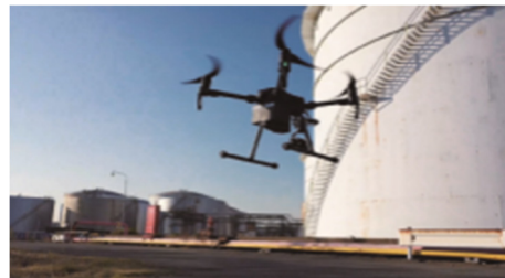
Petroleum tank inspection using a drone
