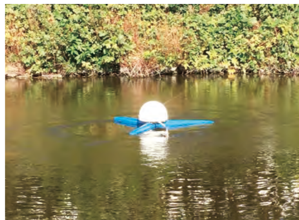
Biofan installed to keep pond water clean
