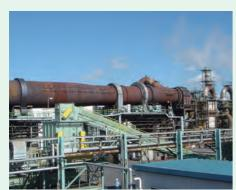
JX Nippon Tomakomai Chemical rotary kiln furnace
