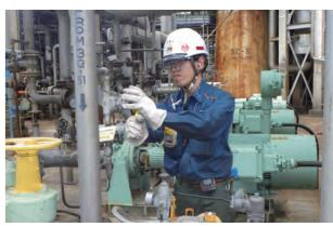
Employee testing for exposure using individual samplers
